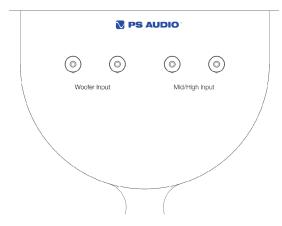
Note: Binding posts may have plugs. If using banana plugs, remove the plugs first.
